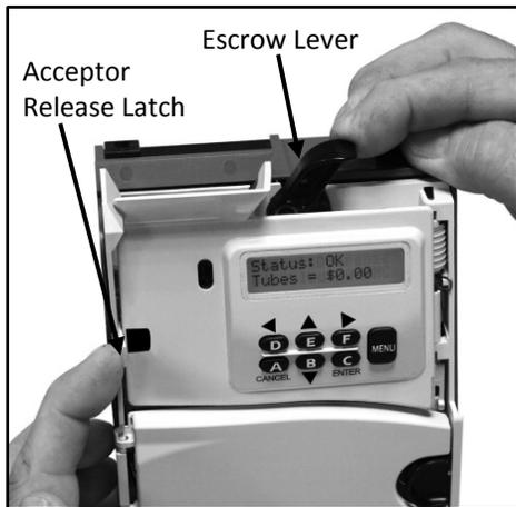
Figure 1. Removing the acceptor.
