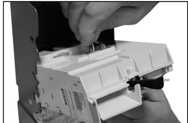
Figure 2. Disconnecting the 2 harnesses.
